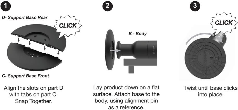
Align the slots on part D with tabs on part C. Snap Together.
